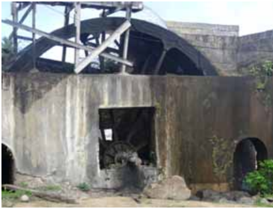
The waterwheel drives the machine that crushes the sugarcane.
