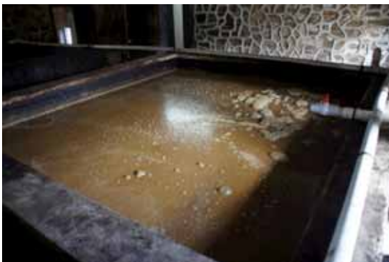
The cold syrup is filled into tanks where it ferments spontaneously. The fermented liquid is then distilled.
