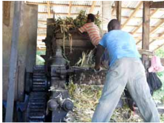
The waterwheel drives the machine that crushes the sugarcane.
