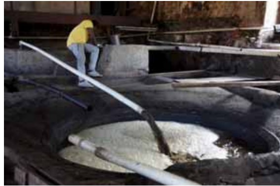
The cold syrup is filled into tanks where it ferments spontaneously. The fermented liquid is then distilled.
