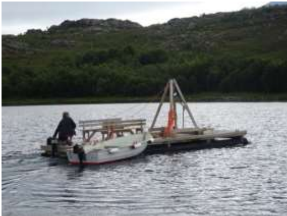
The float is his stone-working vehicle. It's wooden crane above a trap door is designed to transport large stones for the completion of the landing and the
